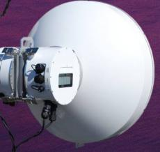
80 GHz 2.50 Gbps Long Range The AireBeam Series provides low latency operation at full duplex Gigabit Ethernet bandwidth, low power consumption at less than 20 Watts, and there are two user selectable antenna configurations for long distance (2 foot/.6m antenna), and medium distance (1 foot/.3m antenna) applications.
