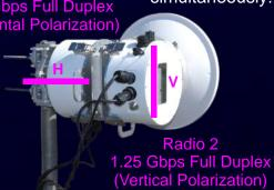
Orthomode Transducer (OMT)
