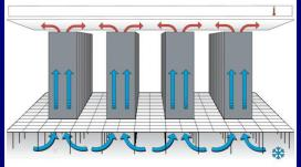
Dust and abnormal humidity are enemies of the electronic devices. To keep the environment at the ideal conditions, a good air condition system is necessary. It provides heat and humidity control, greater airflow and air filtration.
